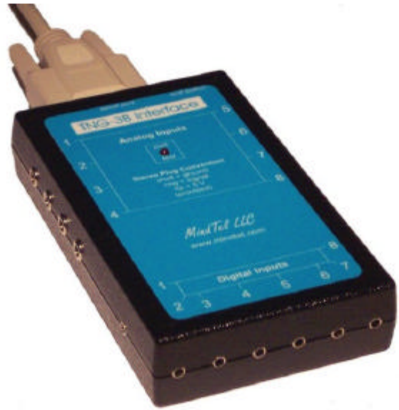
Fig. 2. TNG-3B serial interface.
