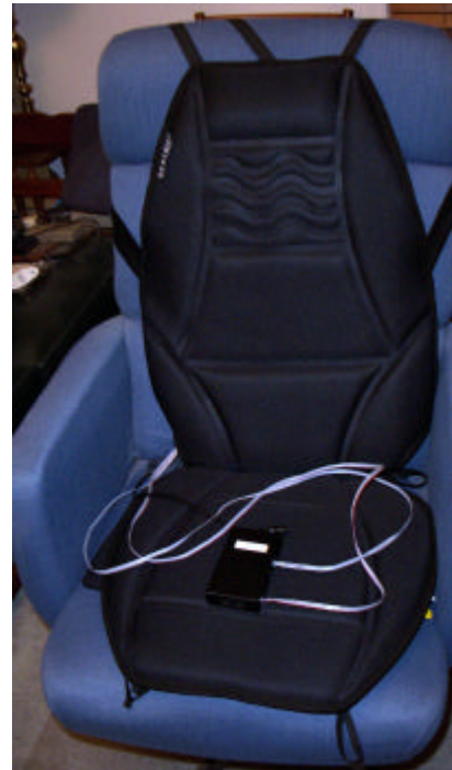
Fig. 16. Modified Homedics 10-motor massage unit.
