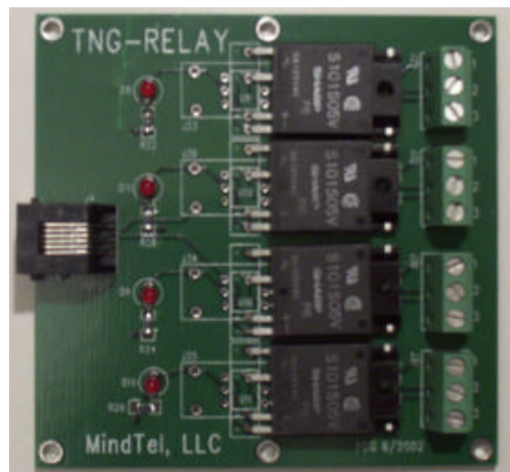
Fig. 14. Relay board with AC relays.
