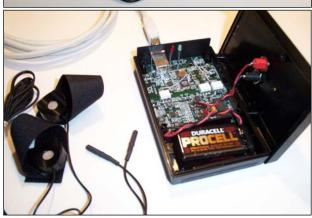
Skin Conductance Module shown with finger electrodes and USB cable. (The box actually has a rear battery door and does not have to be opened as shown to change the battery.)
