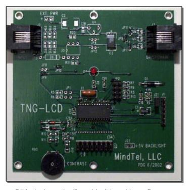
resistors R7, R9, and R3. The jumper adjacent to R7 is the least significant bit of the address. Presence of a shunt constitutes a "1" in the address. The address range is 0-7. Receipt of
