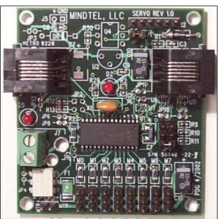
proportional to the duty cycle length of the control pulse. Each motor is sent about 62.5 pulses per second. The pulse width of each motor can be varied from approximately 1 microsecond to 3000 microseconds in 1 microsecond steps. The power-up default is a 1500 microsecond pulse width—the "neutral" position for most servo motors. Most common servos have a hysteresis of 8 microseconds.
