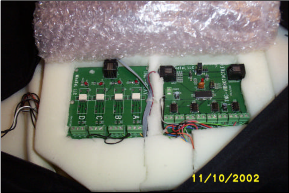
Vibrotactile array driver board along with relay board used to control a massage unit.
